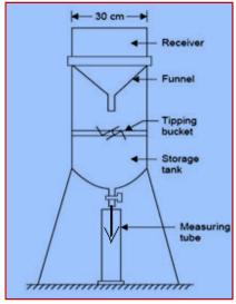
Figure :- Tipping Bucket Raingauge
