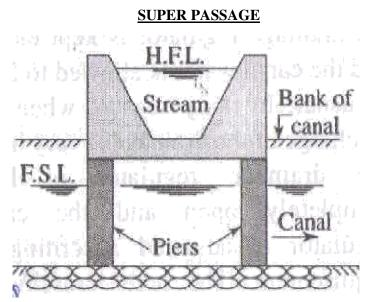
The hydraulic structure in which the drainage is passing over the irrigation canal is known as super passage. It is reverse of an aqueduct. A super passage is similar to an aqueduct, except in this case the drain is over the canal.
