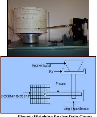
Figure :Weighing Bucket Rain Gauge
