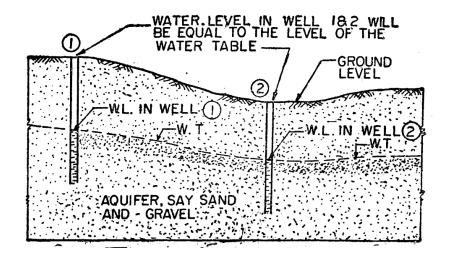
The ordinary gravity wells of 2 to 5 m diameter, which are constructed to gap water from the top most water bearing strata, i.e., from the unconfined aquifers, are known as unconfined or non-artesian wells. The water levels in these wells will be equal to the level of the watertable. Such well are, therefore, also known as wells or gravity wells.
