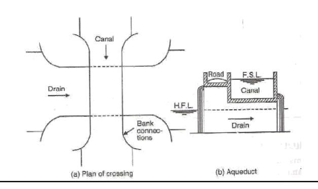
The hydraulic structure in which the irrigation canal is taken over the drainage is known as an aqueduct.
