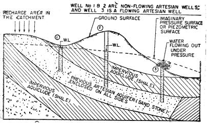
The rains falling in the catchments (i.e., by discharge). However, the water will not rise to this full height, because the friction of the water moving through the aquifer uses up some of the energy.
