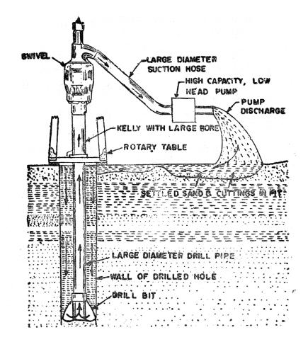
The hole is driven by pumping water under pressure through the drill bit, while it is churned up and down.
