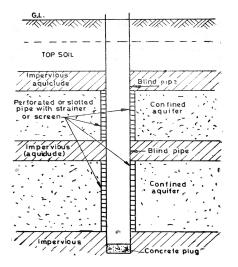
The boring for such a well is generally carried out by a "casing pipe of about 5 to 10 cm larger than the diameter of the well pipe. Thus, for a 15 cm diameter well, a bore hole of 20 to 25 cm diameter shall be drilled. After boring the hole, the well pipe assembly which is partly in ordinary plain pipe (called blind pipe) and partly of strainer pipe, is lowered into the
