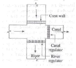
In this type of work, the drainage water is passed into the canal & then taken out at the opposite bank. The work consists of
